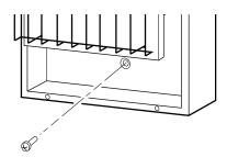
Figure 11 - Installing Bottom Mounting Screw
